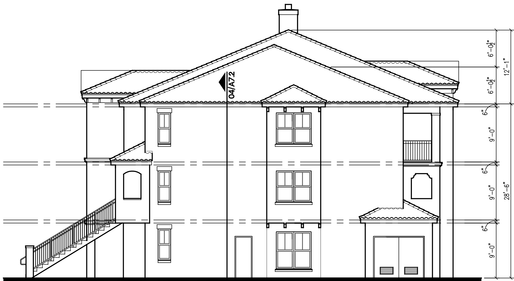
03 BUILDING TYPE II LEFT END ELEVATION SCALE: 1/8"=1'-0" BUILDINGS 9 & 10
