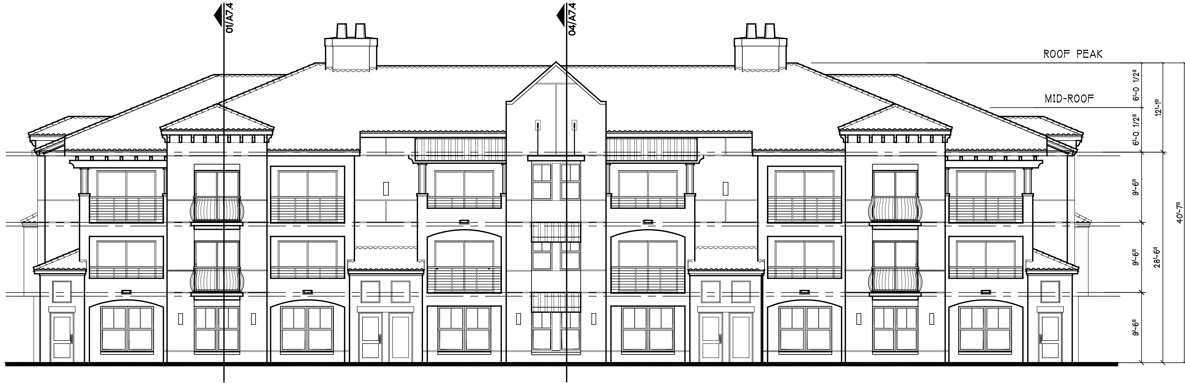
01 BUILDING TYPE IIA FRONT ELEVATION SCALE: 1/8"=1'-0" BUILDING 3
