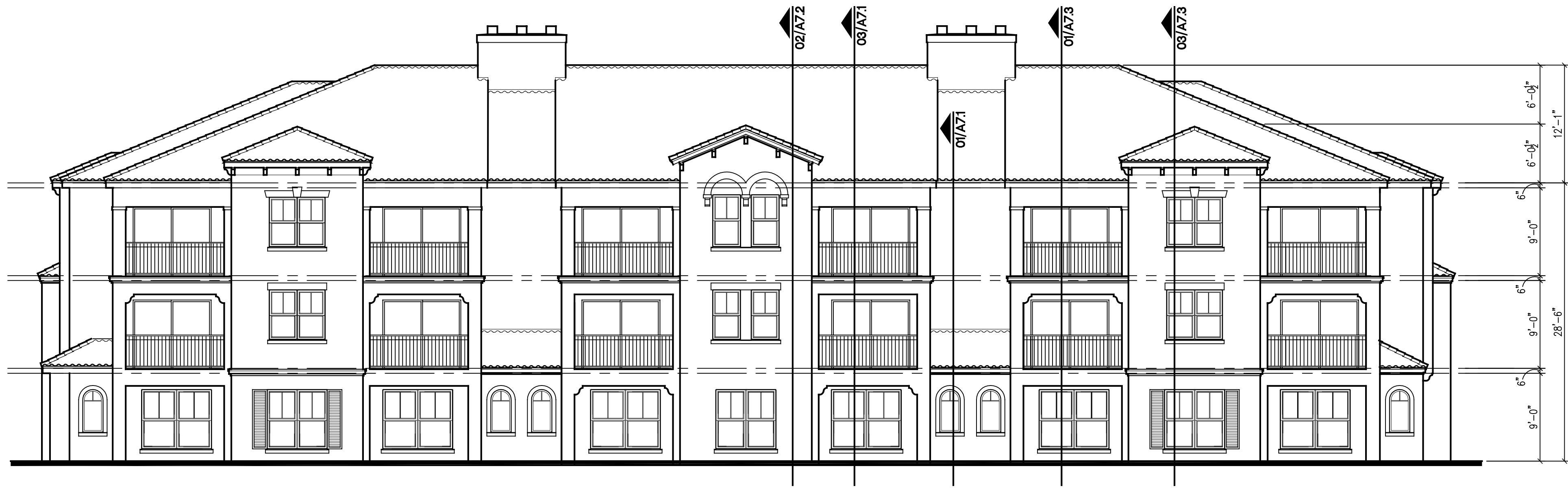
01 BUILDING TYPE II FRONT ELEVATION SCALE: 1/8"=1'-0" BUILDINGS 9 & 10
