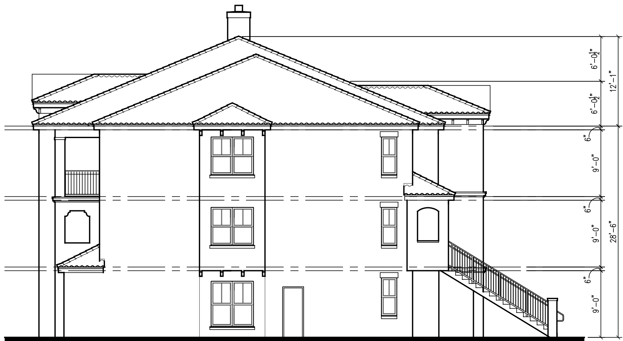
04 BUILDING TYPE II RIGHT END ELEVATION SCALE: 1/8"=1'-0" BUILDINGS 9 & 10
