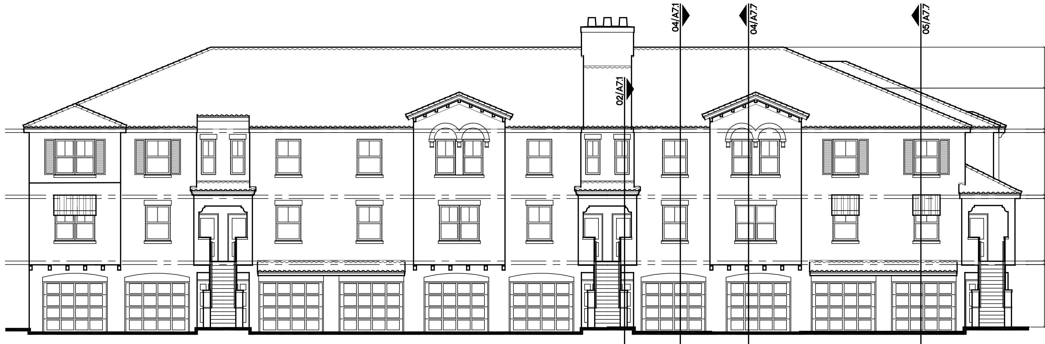
02 BUILDING TYPE III REAR ELEVATION SCALE: 1/8"=1'-0" BUILDINGS 2, 7 & 11
