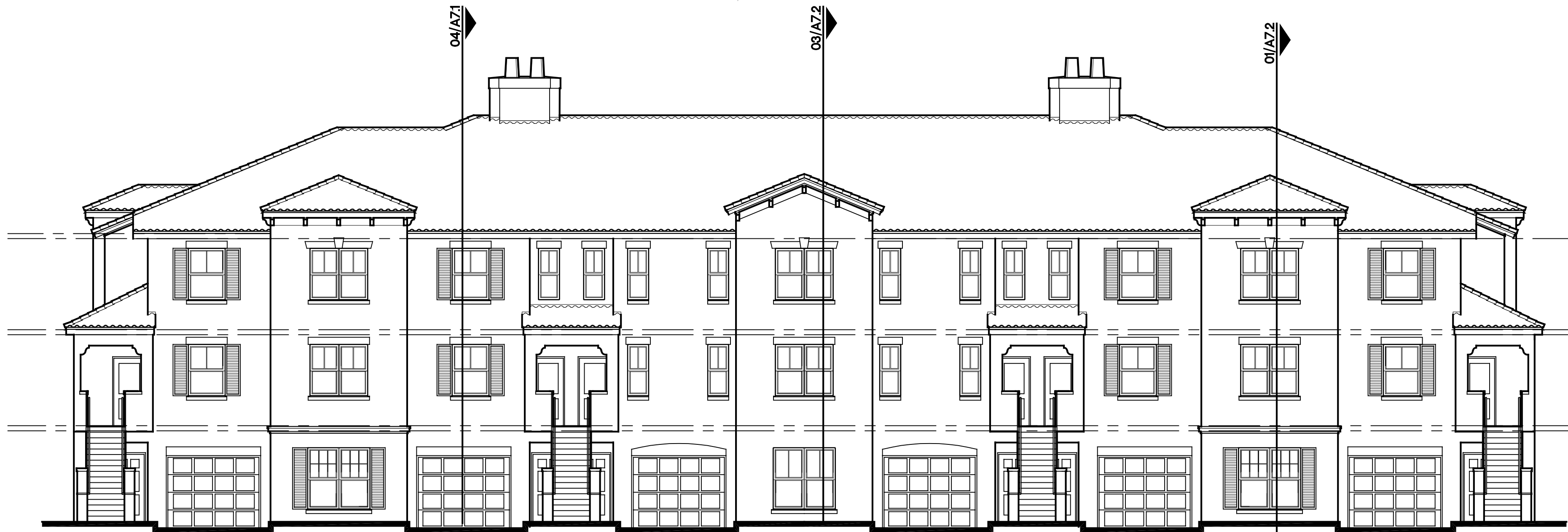
02 BUILDING TYPE IIA REAR ELEVATION SCALE: 1/8"=1'-0" BUILDING 3
