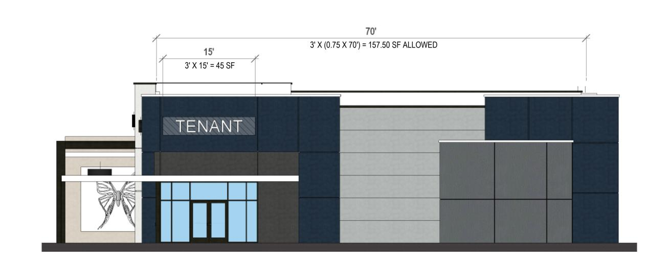
4 BLOCK 3 - BUILDING D - SOUTH ELEVATION SCALE: 1/8" = 1'-0"
