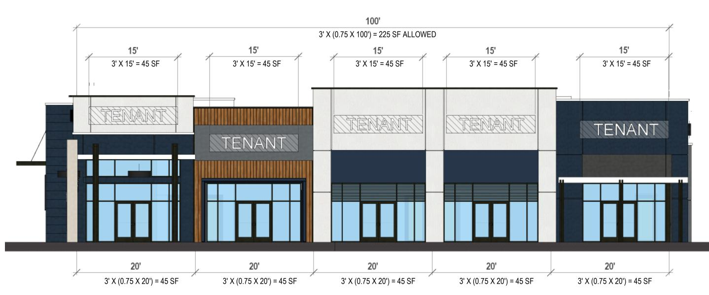
**BLOCK 3 - BUILDING D - WEST ELEVATION** SCALE: 1/8" = 1'-0"
