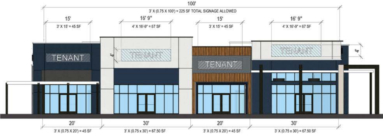
1 BLOCK 3 - BUILDING F2 - WEST ELEVATION SCALE: 1/8" = 1'-0"
