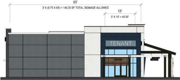
2 BLOCK 3 - BUILDING H - WEST ELEVATION
