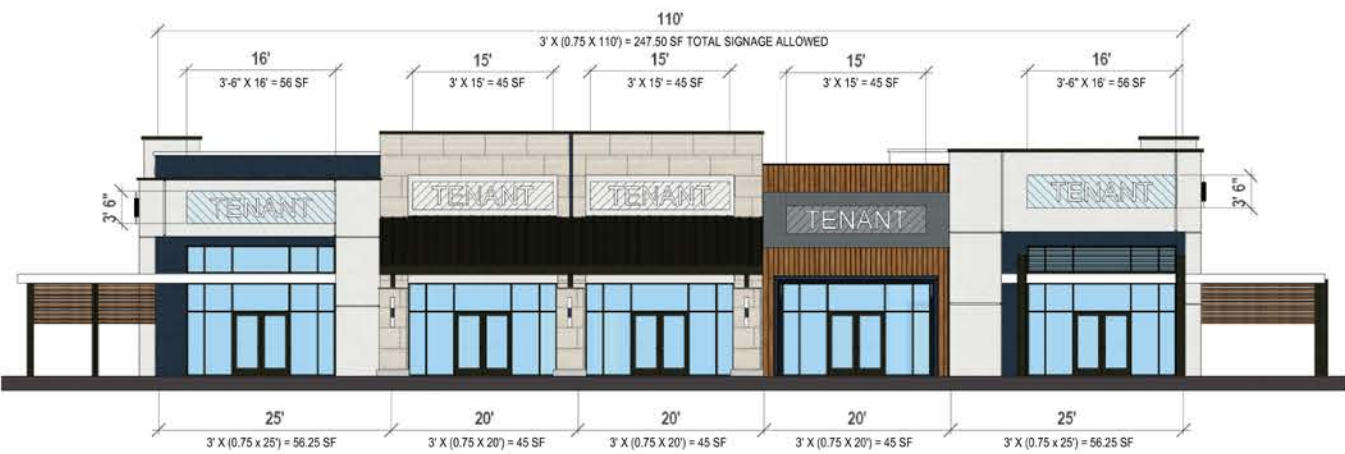
1 BLOCK 3 - BUILDING G - WEST ELEVATION SCALE: 1/8" = 1'-0"
