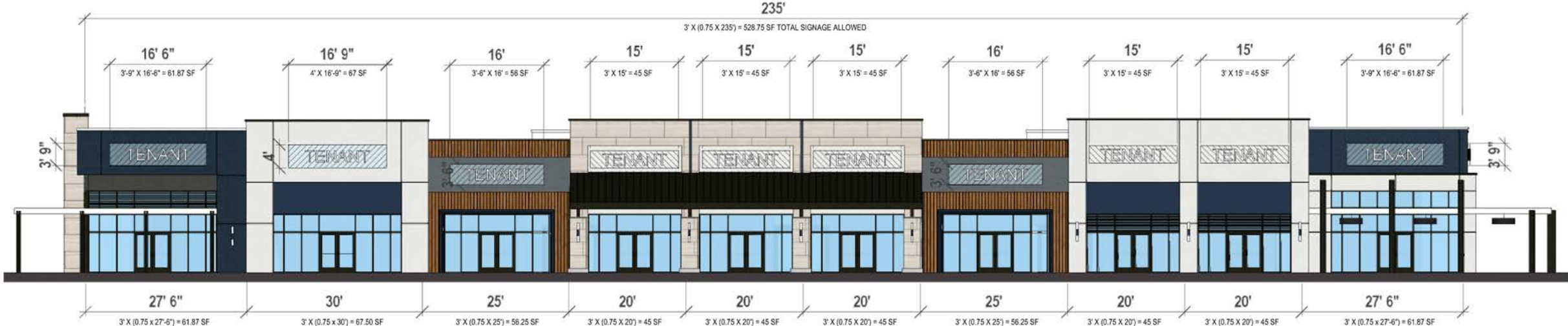
1 BLOCK 3 - BUILDING B/C - EAST ELEVATION SCALE: 1/8" = 1'-0"
