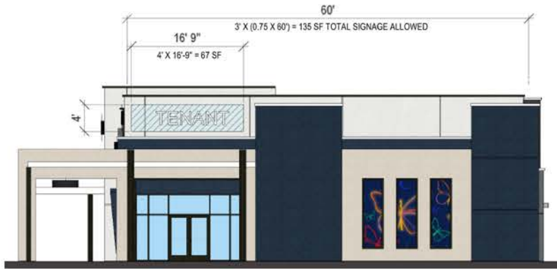
4 BLOCK 3 - BUILDING F2 - SOUTH ELEVATION SCALE: 1/8" = 1'-0"
