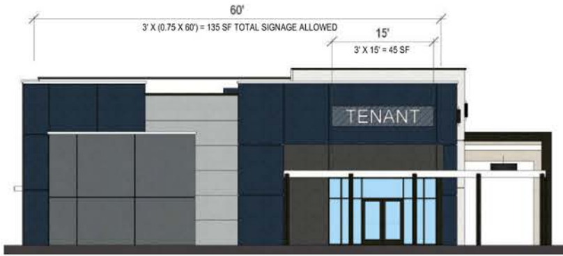
2 BLOCK 3 - BUILDING F2 - NORTH ELEVATION SCALE: 1/8" = 1'-0"
