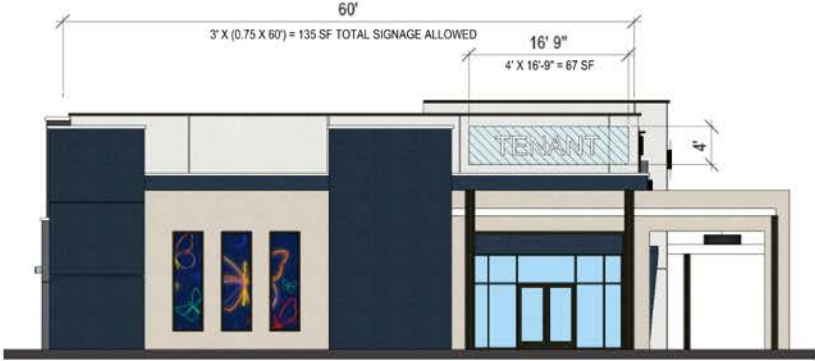
2 BLOCK 3 - BUILDING F1 - NORTH ELEVATION SCALE: 1/8" = 1'-0"
