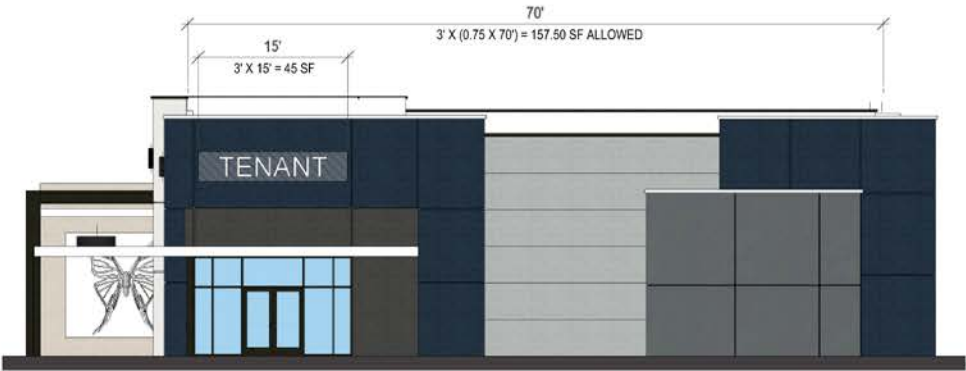
4 BLOCK 3 - BUILDING D - SOUTH ELEVATION SCALE: 1/8" = 1'-0"
