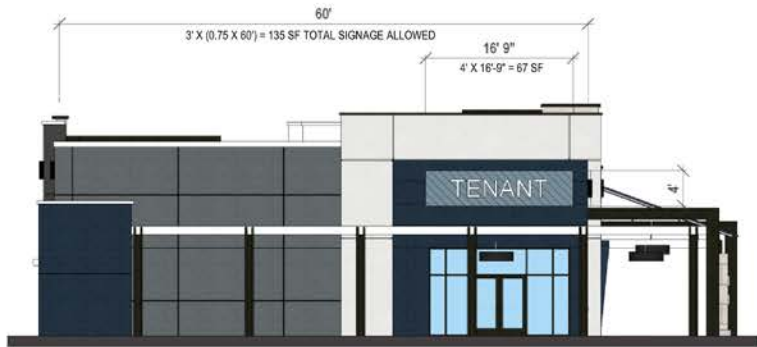
2 BLOCK 3 - BUILDING E - NORTH ELEVATION SCALE: 1/8" = 1'-0"
