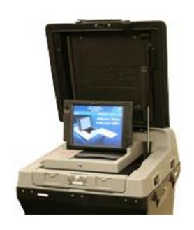
The voter will insert the ballot into the DS 200 optical scanning machine.
