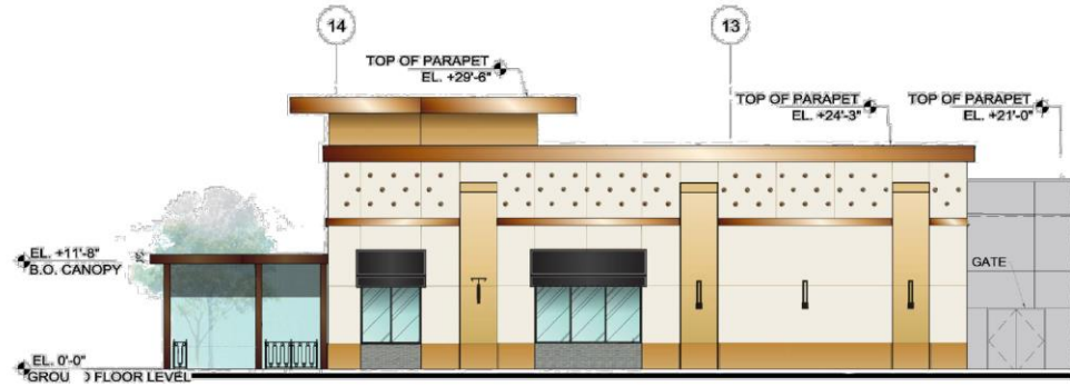
5 PROPOSED WEST ELEVATION A301 SCALE: 3/32" = 1'-0"
